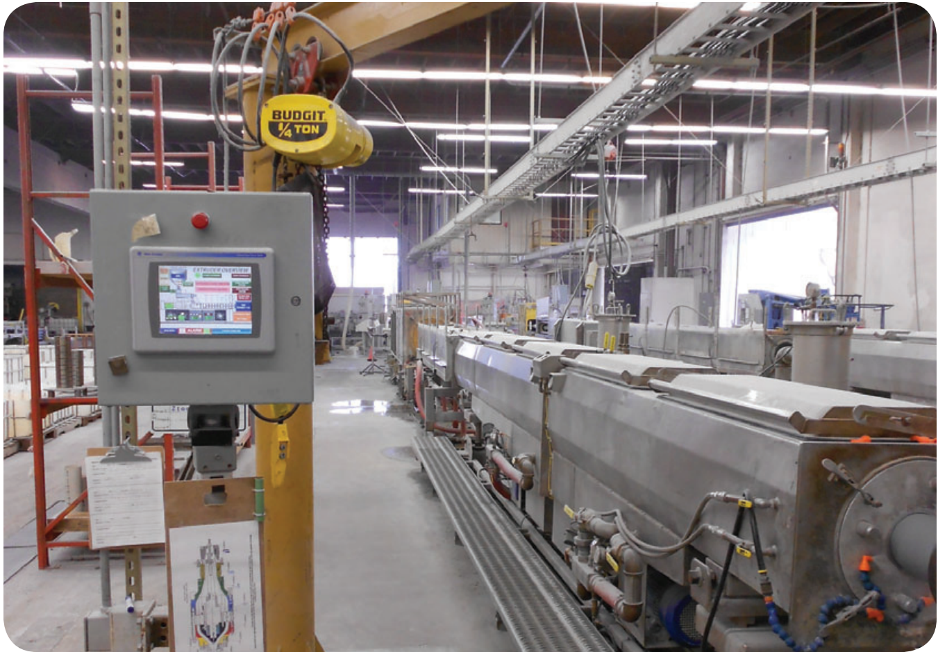
An HMI placed at each end of the four 160-foot extrusion lines allows operators to view any piece of equipment while standing at either end of a line, simplifying maintenance and repair.
